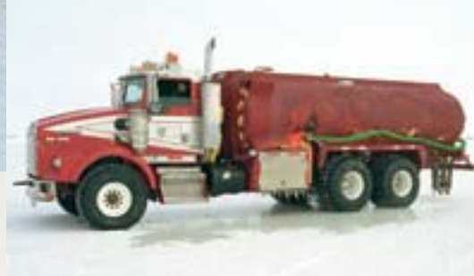
Northwind Industries uses unique equipment, like this water truck, to help build up layers of ice, frozen by the cold temperatures of the Far North.
